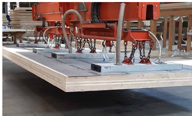
Fast and secure adhesion
