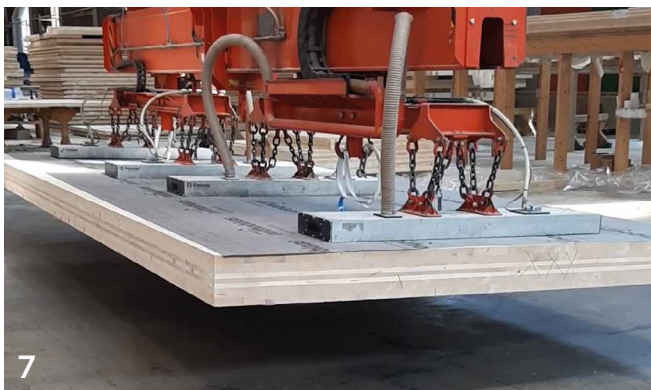
7 Suitable for vacuum lifting systems.
