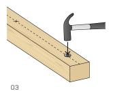
Use a hammer to insert the bushing.
