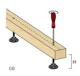
Adjust the height of the support from above using a flat screwdriver.
