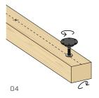
Screw the support into the bushing and turn the joist.
