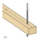
Trace the joist midline, indicating the position of the holes and then pre-drill a 10 mm diameter through hole.
