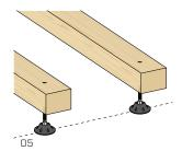
Place the joist on the substrate, parallel to the one previously laid.
