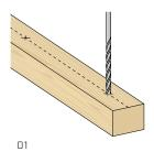
Trace the joist midline, indicating the position of the holes and then pre-drill a 10 mm diameter hole.
