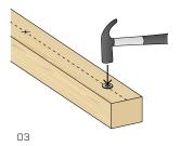
Use a hammer to insert the bushing.
