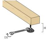
Adjust the height of the support from the bottom using a 10 mm SW wrench.
