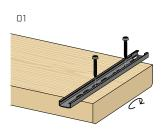
For each board arrange one fastener and fix it by means of two KKTX screws.
