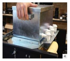
Position the colour tank and make sure that nozzles are closed. Hook the collection bucket under the tank.
