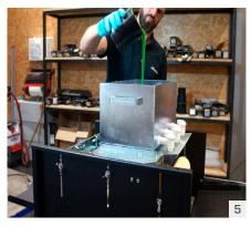
Enter paint or impregnating primer. If necessary, mix it until a homogeneous consistency is obtained.
