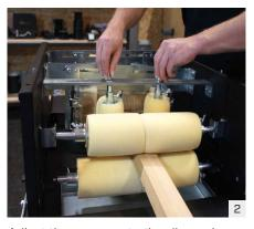
Adjust the sponges to the dimensions of the element and fix them by tightening screws.
