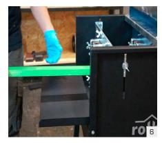
Start the process: open the nozzles and wait for the rolls to absorb the colour. Finally, push the elements through the sponges.
