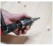
Turn the outer sleeve to reset the TORQUE LIMITER.
