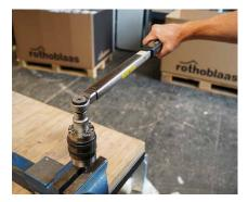
Perform an initial torque check with a torque wrench.
