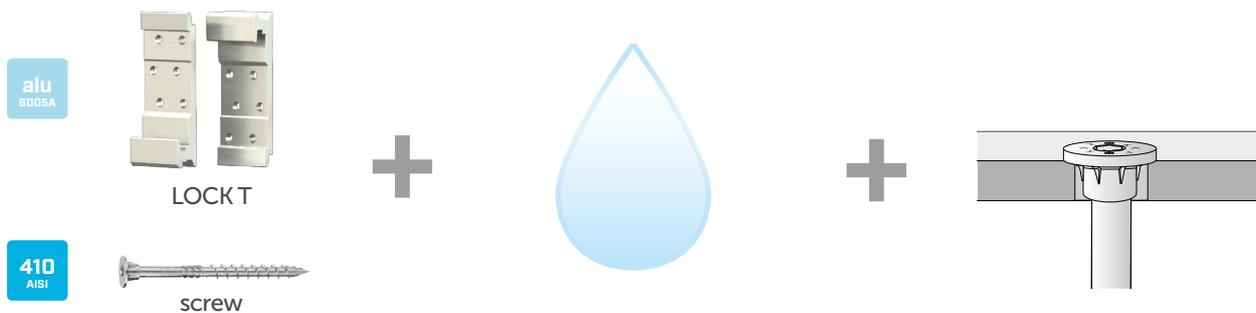
This is effectively solved by the LOCK T EVO version with polyester powder coating, which electrically insulates the parts and thus prevents galvanic corrosion. With this solution, a longer life and reliability of the LOCK T connectors is guaranteed, even in humid environments.<sup>(1)</sup>
